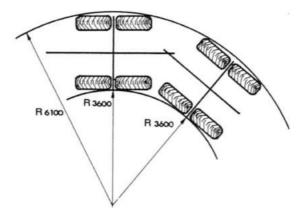
Fig. 3. The turning radii and travelling width of the Bruunett mini 578 F forwarder (measurements in mm)
