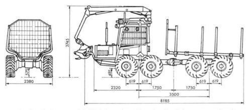
Fig. 2. The Bruunett mini 578 F forwarder. Dimension sketch (measurements in mm)
