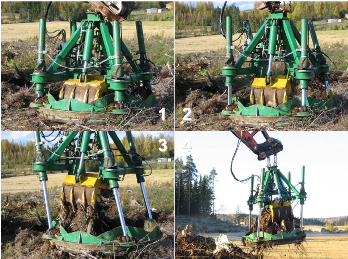
Figure 3. The work cycle of the Järvinen stump-lifting device.
