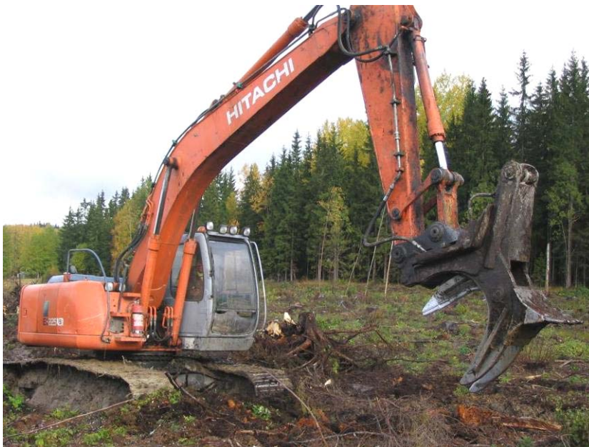
Figure 4. Hitachi EX 225 USR tracked excavator equipped with the Väkevä Stump Processor lifting head in the time study.
