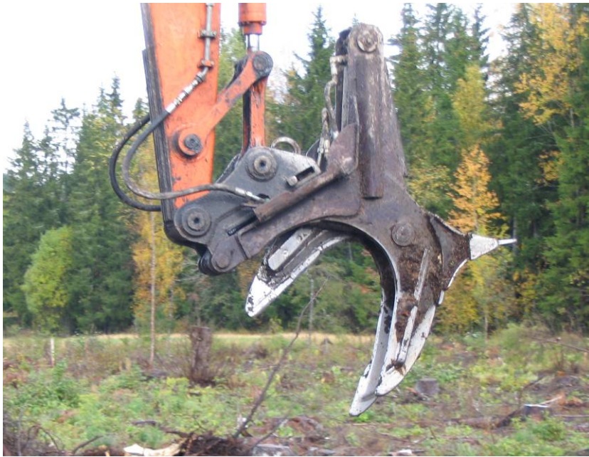
Figure 2. The Väkevä Stump Processor lifting head tested in the time study. Photos: Kalle Kärhä / Metsäteho Oy.
