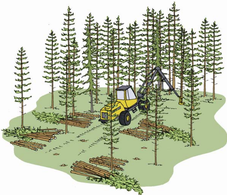
Figure 1. The integrated wood procurement system based on the two-pile method, in which pulpwood and energy wood fractions are stacked into separate piles in early thinnings. Drawing: Juha Varhi, © Metsäteho Oy.
