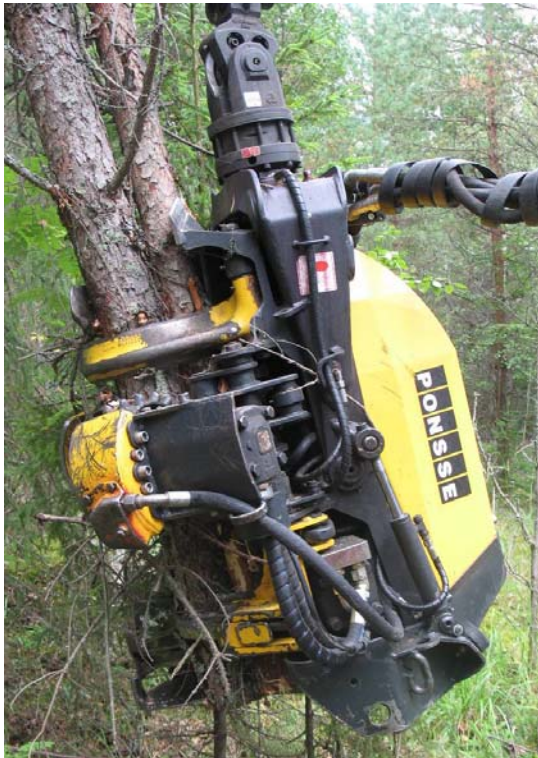
Figure 2. The new Ponsse H53e harvester head with a multiple-tree processing property. Photo: Kalle Kärhä, Metsäteho Oy.
