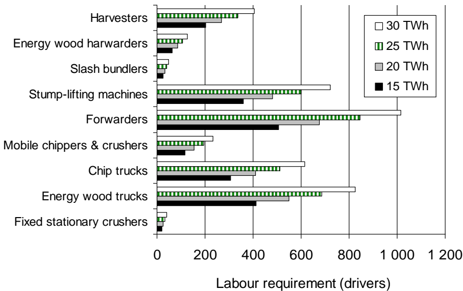
Figure 6. Estimated machine and truck driver requirement for forest chip production by machinery type in 2020, if the production and usage of forest chips is 15 to 30 TWh.
